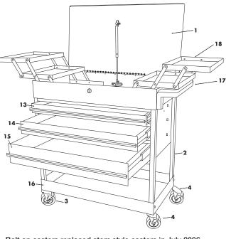
Bolt on casters replaced stem style casters in July 2006. If your MB155UC has stem style casters contact Mac customer service for caster and bottom shelf part numbers.
