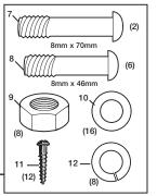
Bolt Kit (#6) included for attaching legs and tray to MB155UC cart:
