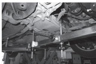
Position the two central hooks on either side of the engine cradle. In certain cases, one hook only can be positioned.
