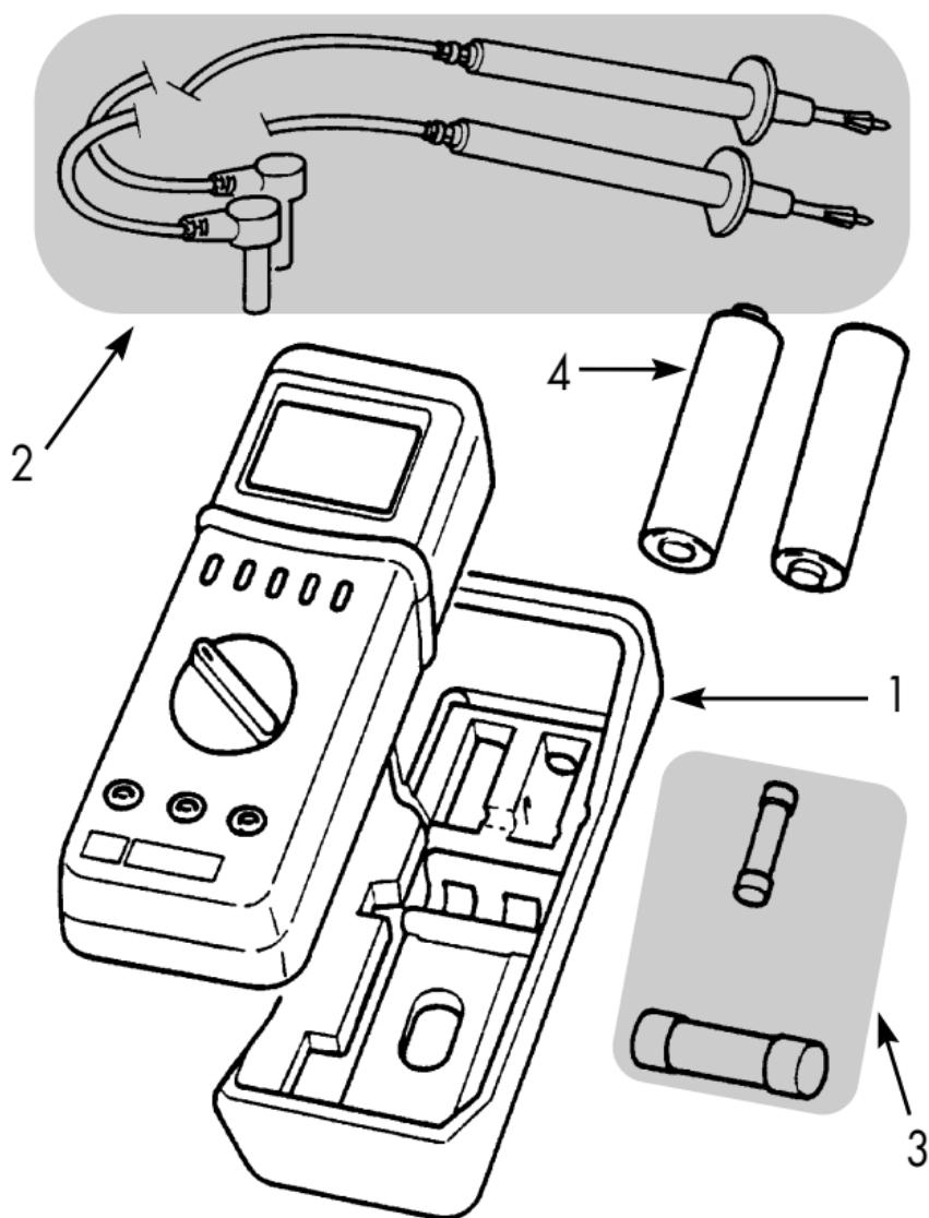
To replace the batteries or the fuses, remove the 3 screws from the detachable part of the rear case of the tester.
