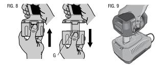
To install the battery pack into the tool handle, align the notch inside the tool's handle with the battery pack and slide the battery pack firmly into the handle until you hear the lock snap into place as shown in Figure 8.
