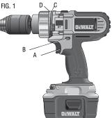
The center position of the control button locks the tool in the OFF position. When changing the position of the control button, be sure the trigger is released. **NOTE:** The first time the tool is run after changing the direction of rotation, you may hear a click on start up. This is normal and does not indicate a problem.
