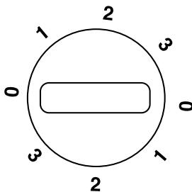
This can be operated by pulling the head string as well with every pull the switch advances to the next level of operation from 0-1-2-3 back to 0.
