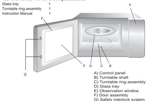
Shut off oven power if the door is opened during operation.
