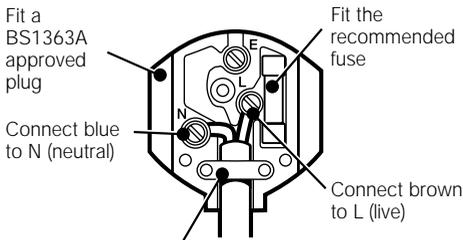
Make sure that the outer sheath of the cable is held firmly by the clamp
